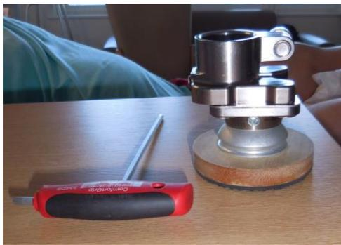
Loading device for attachment to a bone-anchor.
